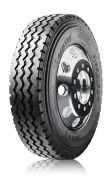
The S812's unequal pitch of tread patterns is designed to reduce the rolling noise of the tyre. The bead reinforcement technique provides excellent load resistant power. Its closed shoulder is used both to guarantee its good stability and reduce the abnormal wear of its shoulder.
