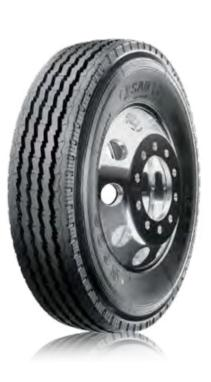
The S626 is designed with tread rubber, with low heat generating qualities, with excellent burst and abrasion resistance . Using the design of four longitudinal grooves with good drainage, even distribution of ground contact pressure, prevention of irregular wear and tear, and superior manoeuvrability and comfort.
