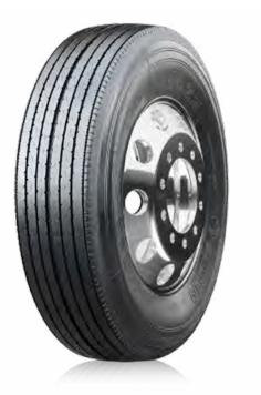
The S622 is a premium free-rolling position trailer tire. With a decoupling groove that resists irregular sidewall wear, and wide ribs to prevent damage caused by high-scrub applications. The S622 is also a low-rolling resistance tire designed to maximize your mileage.
